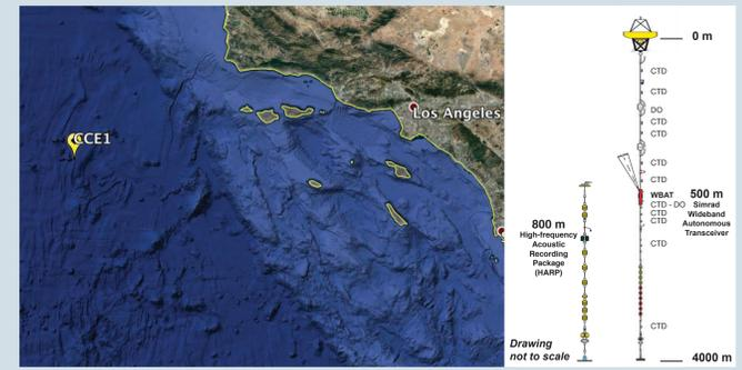
Figure 1. Left: Location of the California Current Ecosystem mooring 1 (CCE1) offshore Southern California in 4000 m water depth. Right: Mooring drawings with passive and active acoustic recorders and CTDs.
